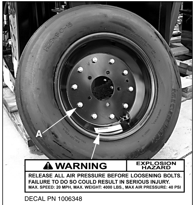
Figure 19. Split Rim Tire Servicing
